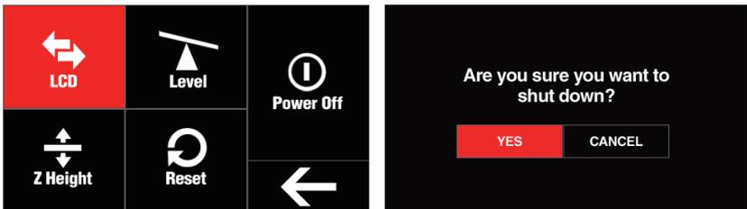
**Power Off:**You can shut down D7 Plus. This will not power off the printer.
