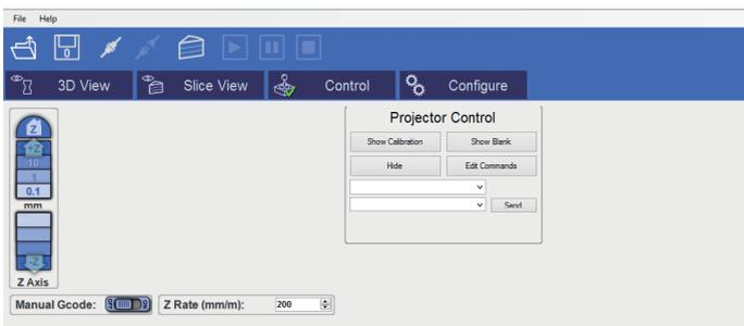
From this screen we will be able to control the motors of the printer , which means displacing the build base over the Z axis, as well as controlling the LCD.
