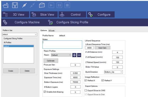
In order to slice a model into images, you must first set up a slicing profile. A default profile has been created the first time the application was started. You can create new slicing profiles and manage them in much the same way you can manage machine profiles. The ‘Slice Profiles Config’ tab item will allow you to create, delete, or edit a slicing and building profile.
