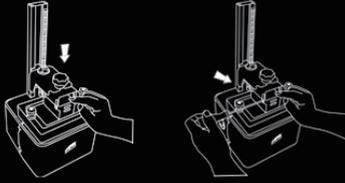
After homing, press down the platform to touch the FEP film with one hand. Tighten the 4 screws by the other hand.
