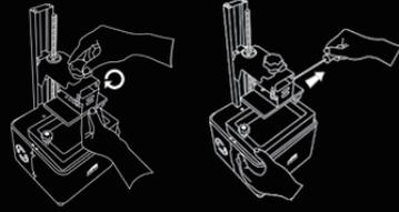
**Tighten the central knob and loosen the 4 screws, so the platform can move up and down freely. Then click Next.**
