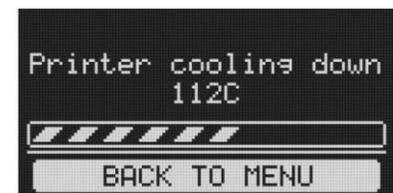
14. Once the cool down process has finished, you can remove the print from the build plate. The best way to do so is with the included scraper.
