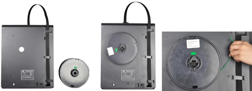
4. Select the **Move material** option. Wait for the nozzle temperature to reach the target value (200°C).
