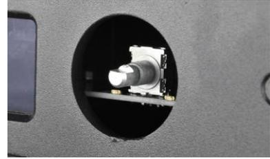
16. Position the control knob with the locking screw facing up, then slide it onto the control post.
