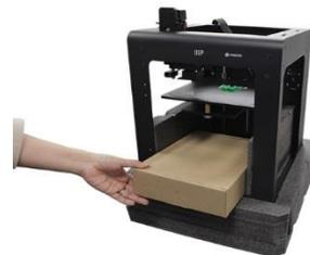
10. Fold the protecting foam and carefully pull it out from under the print bed.
