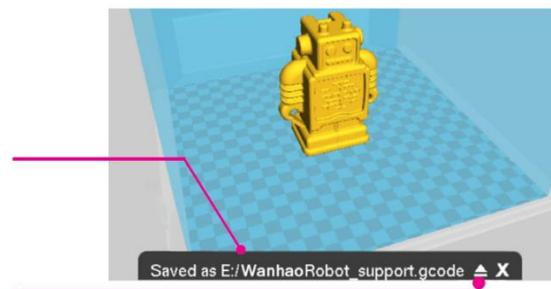
9. Ensure that the printer is powered off, then insert the SD card with your saved file into the SD card slot to the left of the display on the front of the printer. Power the printer on.
