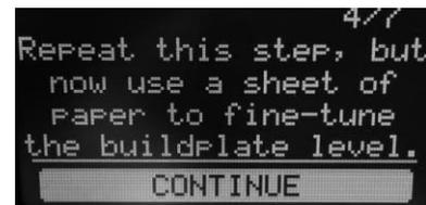
8. The extruder will move to the center front of the build plate. Adjust the screw under the center-front until you can move the paper with a slight bit of resistance. Select the **CONTINUE** option to proceed.
