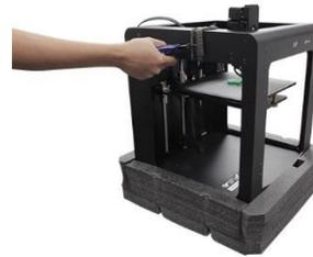
12. Carefully lift the printer out of the foam cradle and set the foam aside.
