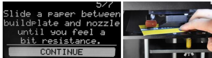
9. The extruder will move to the left-rear of the build plate. Adjust the screw under the left-rear corner until you can move the paper with a slight bit of resistance. Select the **CONTINUE** option to proceed.
