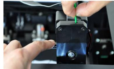
6. Turn the control knob clockwise until your filament starts to extrude out of the nozzle. Note that the initial material coming out of the nozzle may not be the same color as your filament. This is because factory testing of this printer may have left some residual filament in the nozzle. Keep turning the control knob until the correct color material starts to extrude. Press the control knob to continue.
