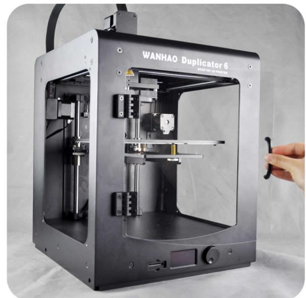
9. Fix the side cover with the 4mm hex wrench and M5\*10 screw.
