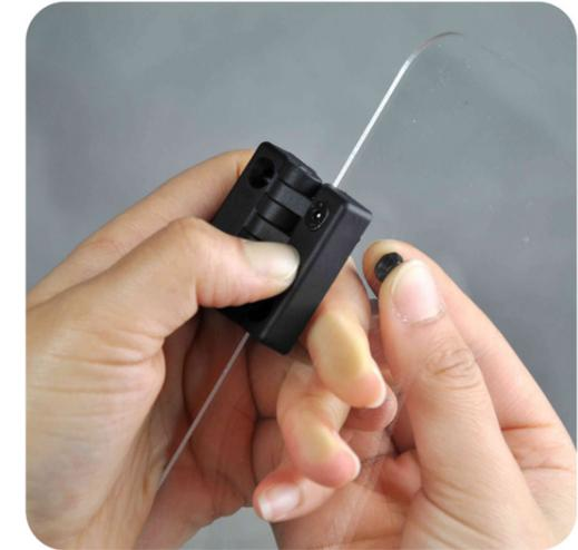
5. Use M4\*5 screw and 3mm hex wrench to fix the handle on the front cover. In this step, you need two M4\*5 screws.
