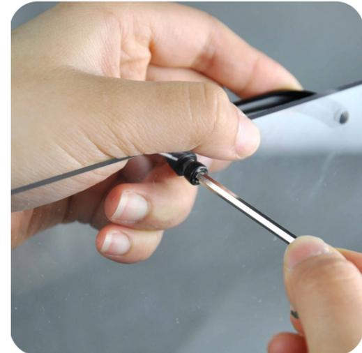
6. Fix the front cover on the printer with the 2.5mm hex wrench and another four M4\*16 screws.
